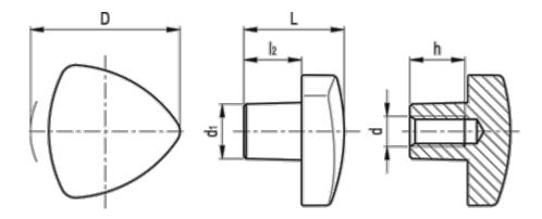
$\begin{array}{lll} D & = 32 \\ d & = M5 \\ d1 & = 12 \\ h & = 10 \\ L & = 21 \\ l2 & = 12 \\ Weight (g) = 60 \end{array}$
